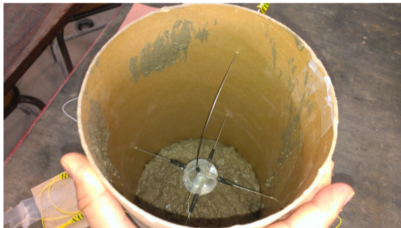
Sensor put in concrete
